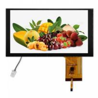
Gray Scale Inversion Direction: 6 o'clock Interface: 24bit parallel RGB interface
