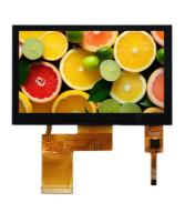
The CH430WQ12A1-CT has dimensions of 105.5\*67.2\*4.95 mm, a display area of 96.0454.86 mm, and an active area of 95.04\*53.86 mm. The module consists of a TFT LCD panel, a capacitive touch panel, a driver IC, a backlight, and an FPC. It supports a 24-bit parallel RGB interface and an I2C touch panel interface. Its operating temperature range is -20 to +70, and its storage temperature range is -30 to +80, ensuring reliable performance in harsh environments.
